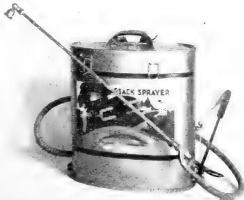
FIGURE 162.—Knapsack sprayer. Useful for large gardens.
