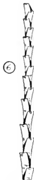
VIEW OF CUTTING EDGE OF RIP SAW FROM ABOVE AND AT AN ANGLE.
