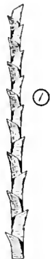
VIEW OF CUTTING EDGE OF CROSSCUT SAW FROM ABOVE AND AT AN ANGLE.
