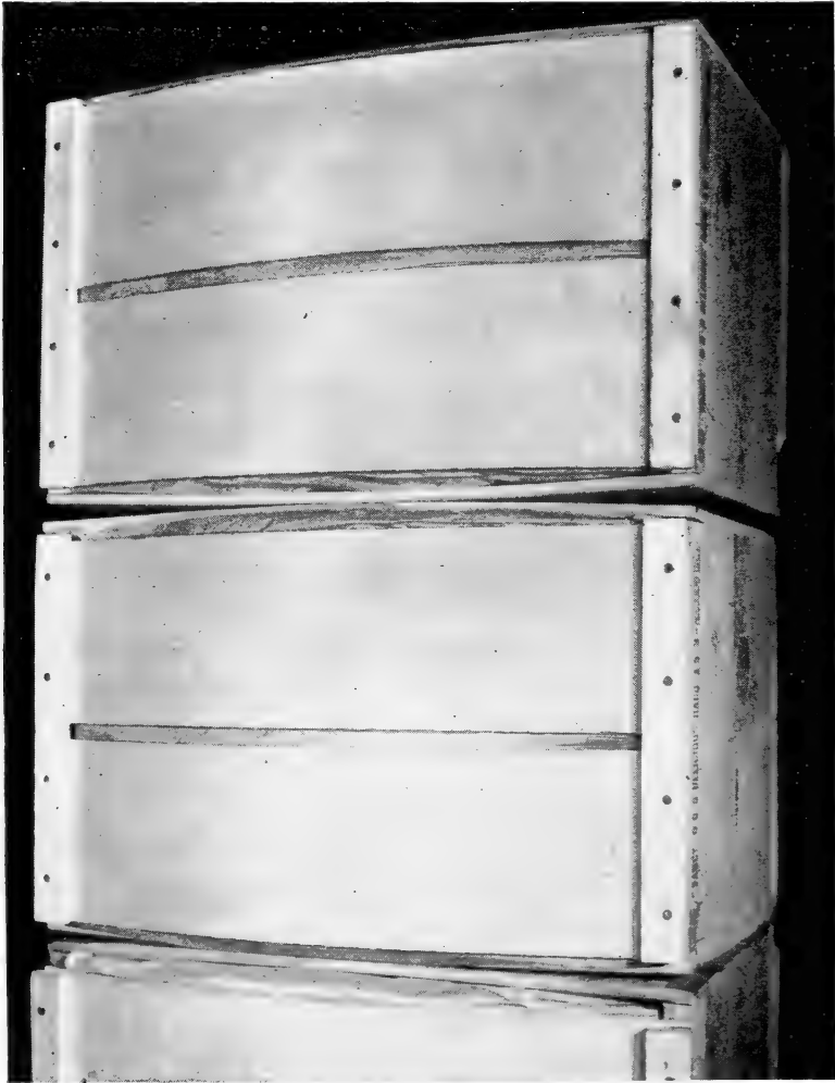
FIGURE 15.—Bulging of top, bottom, and sides of standard boxes because of overfilling. When such overfilled boxes are put under pressure in a stack serious bruising results on apples in contact with the sides and the lids.
