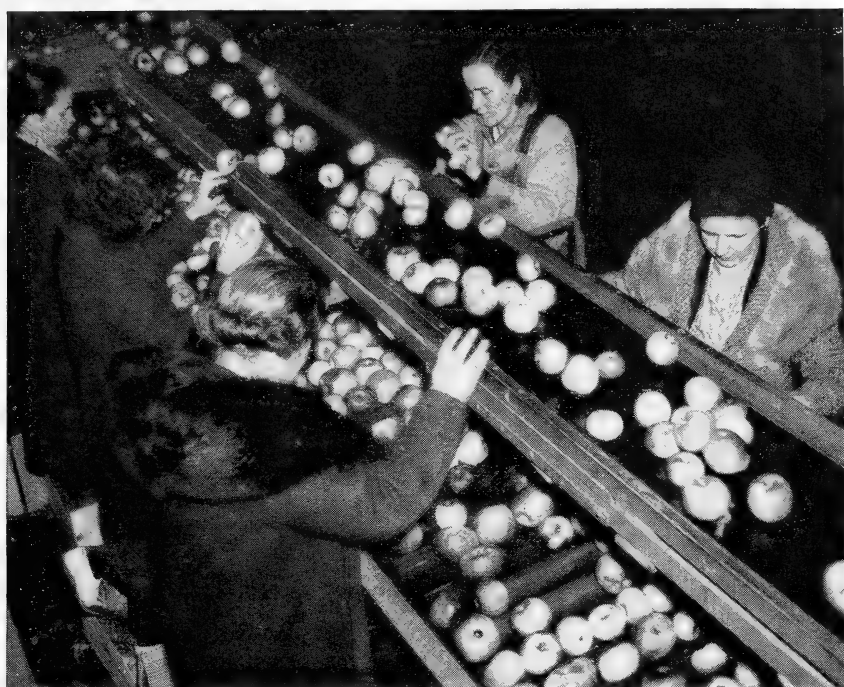
FIGURE 10.—Use of adequate grading and sizing machinery, an important factor in the reduction of bruising. All the sorters should wear gloves.
