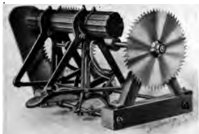
Fig. 51. Combination Lath-Binder and Trimmer. With this machine the operator can trim the bundles of lath, simply by tilting the packing frame over from him causing the bundles to pass between the saws, thereby trimming both ends at one movement.
