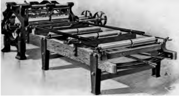
Fig. 43. Double Gang Edger. This machine trims off the rough edges of the "waney" boards by means of the four saws in the main frame of the machine.
