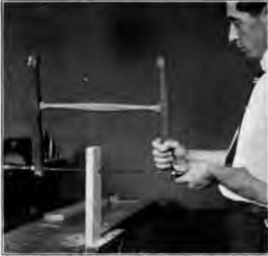
Fig. 95. Using a Turning-Saw.
