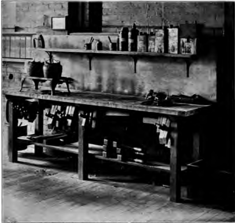
Fig. 243. Gluing and Staining Bench Covered with Zinc.
