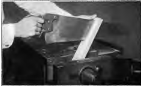
Fig. 89. Rip-sawing with Wood Held in Bench-Vise.
