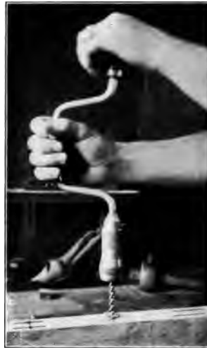
Fig. 263. Boring for Dowels in an Edge-to-Edge Joint.
