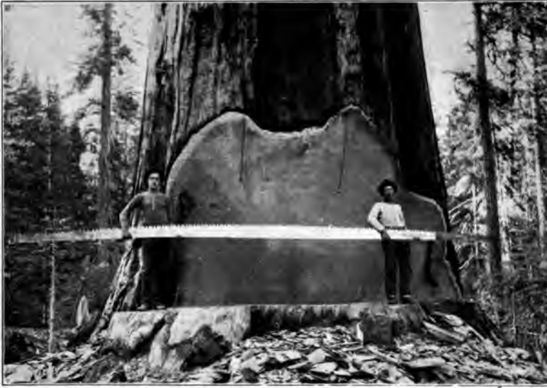
Fig. 25. A Twenty-Five Foot Saw used for Crosscutting Big Logs.
