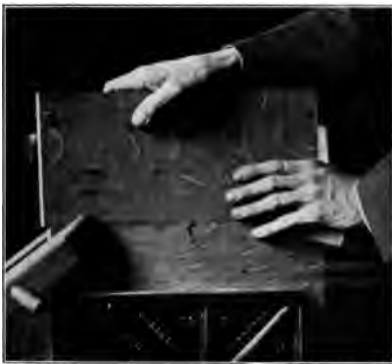
Fig. 261. Rubbing a Glued Joint.
