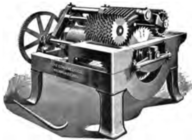
Fig. 49. Ten Saw Gang Lath-Bolter. This machine cuts up material lengthwise into laths.
