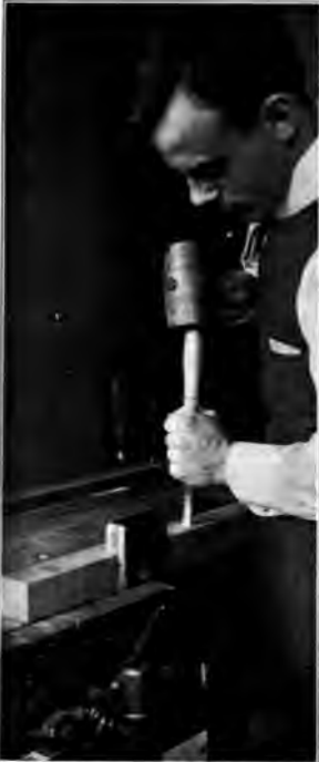
Fig. 76. Mallet Chiseling. The Piece is Clamped Down on the Bench With the Bench-Hook.
