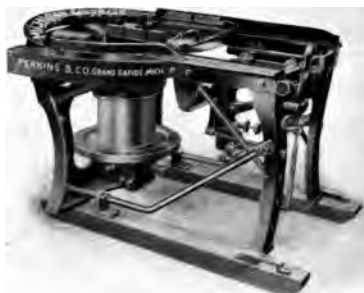
Fig. 52. Hand Shingle-Machine. This machine is used in Sawmills in which it is desired to utilize slabs and trimmings by sawing shingles therefrom, or to saw shingles from prepared bolts.
