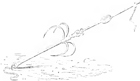
Fig. 36.—Position of grapple after being freed by the breaking of safety-line.
