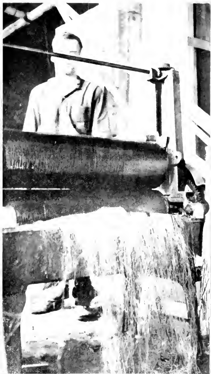
WHAT GOOD IS A TEST RUN? THE ILLUSTRATION SHOWS HOW GLUE MAY BE WASTED IN EVERY DAY WORK. THIS CONDITION DOES NOT APPEAR IN TEST RUNS.
