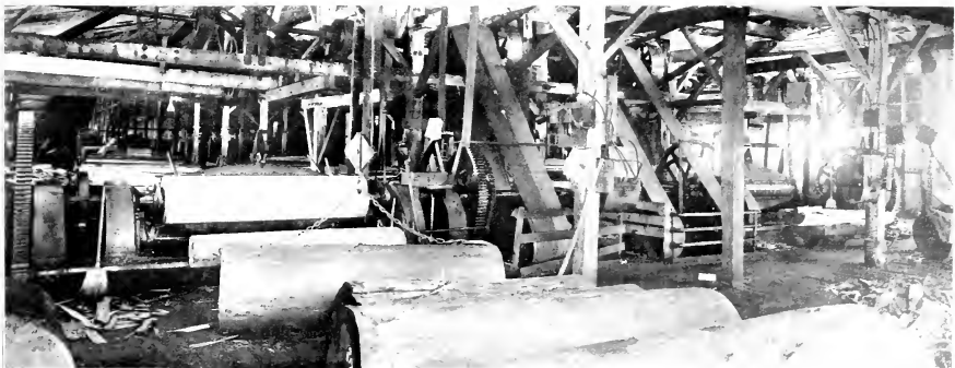
CUTTING ROOM OF THE VENEER PLANT AT WEST HELENA, SHOWING TWO 10-INCH ROLLERS
