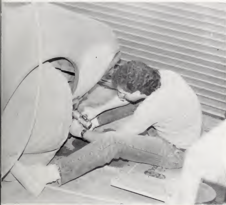
Kevin Holbrook takes extra care to get parts off the car that doesn't need painting.
