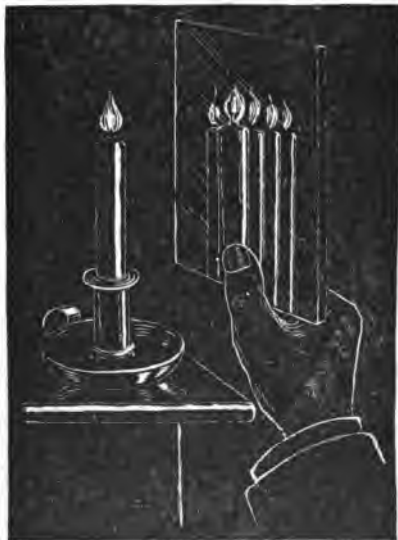
FIG. 3,774. —Experiment illustrating multi-image in ordinary mirror. Let the flame of a candle be observed very obliquely in an ordinary mirror. From four to ten images of the flame may be seen arranged in a row, as here shown. The second image of the series will be by far the most brilliant.
