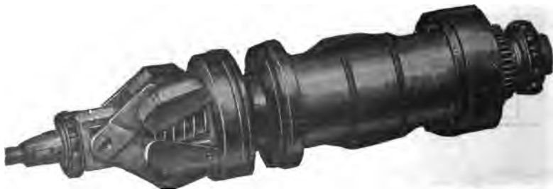
FIG. 3,981.—Automatic spark advance mechanism and armature of Eisemann magneto. The automatic advance is accomplished by the action of centrifugal force on a pair of weight attached at one end to a sleeve through which runs the shaft of the magneto, and hinged at the other end of the armature. Along the armature shaft, run two helicoidal ridges which engage with similarly shaped splines in the sleeve. In operation , the rotation of the armature causes the weights to spread and exert a longitudinal pull on the sleeve which in turn changes the position of the armature with reference to the pole pieces. Thus, the moment of greatest induction is advanced or retarded and with it the break in the primary circuit, for the segments (or cams) which left the circuit breaker and cause the break in the primary circuit are fixed in the correct position and thus the break occurs only at the moment when the current in the winding is strongest. On other magnetos it is the segments or cams that are moved forward or back as the case may be. To apply the automatic control principle to any engine, there have been produced spindles of varying pitches; spindles that will give 19, 25, 38, 45 and 60 degrees advance. For use in connection with these spindles, there are sixteen different springs. With these parts, in connection with the governor mechanism, 160 advance curves can be produced. By varying the length of the stop on the bronze nut, more may be obtained. Many engines require a great deal of advance, others will not permit of more than 20 to 25 degrees. It is necessary to take into consideration the size and shape of the combustion chamber, the compression, the position of the spark plugs and the speed of the motor. It is also universally acknowledged that an engine of high compression will give a quicker burning mixture and will not require, or in some cases, stand, as early a spark as one of lower compression.
