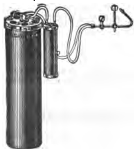
FIG. 3,861. —Fulco pastil adapter. By means of this device the Guil pastil may be used with any calcium burner. The main portion of the adapter is a hollow shell which serves as a receptacle for the pastil when not in use.
