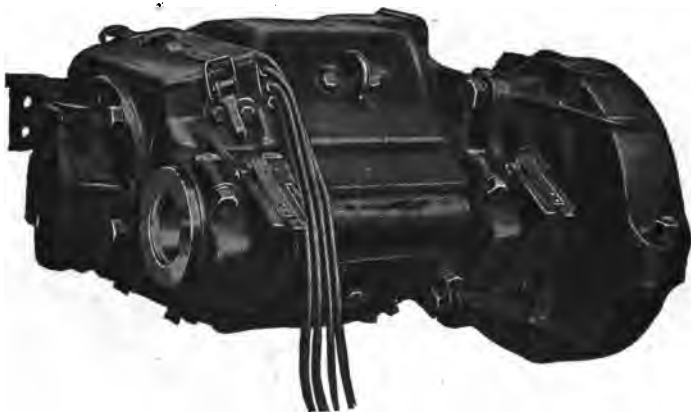
FIG. 3,517. —General Electric standard box frame motor. In this type the magnet frame is one piece of cast steel, and, as shown, is approximately octagonal in shape. The frame is provided with bored openings at each end, through which the armature, pole pieces, and field coils can be inserted or removed through the pinion end opening. Bails are cast on the frame at convenient points to facilitate handling. The opening through the frame over the commutator is large and inclined at an angle to allow easy access to the commutator and brush holders. Hand hole openings are located at points most convenient for the inspection of the interior of the motor. Drain holes are drilled in the lower side of the motor frame. The axle caps (which are inclined at an angle of approximately 60 degrees to the horizontal) are tongued and bolted to machined surfaces on the magnet frame.
