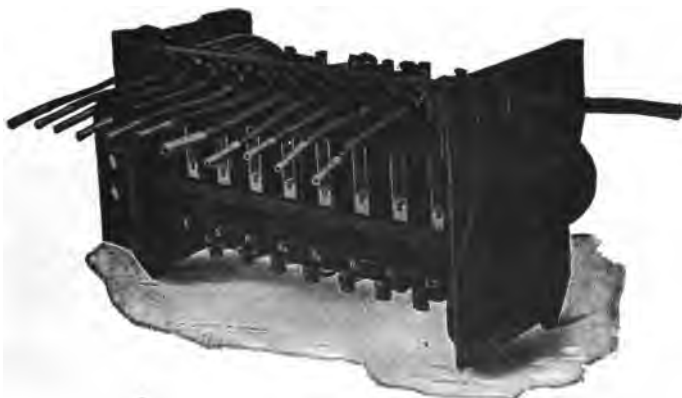
FIG. 3,640.—Westinghouse switch group, covers removed, front view. The most important item of a control equipment is the switch group. This consists of a cast and malleable iron frame upon which the various switches are mounted, completely enclosed by three easily removable sheet iron covers. A blow out coil is located at the side of each switch in order to extinguish the arc formed when the switch is opened under load. The motor cut out switches and the control circuit terminal board are located in a suitable compartment on one end of the group and the overload trip, when not mounted on a line switch, is on the other. The term unit switch as applied to this system of control signifies that the fundamental pieces of apparatus have all parts arranged on the unit plan, so that any worn, or damaged part may be removed and replaced. A switch group, for instance, is made up by assembling the requisite number of each of four different units, known respectively as the switch , the cylinder , the magnet valve and the blow out coil , these being described in the accompanying cuts.
