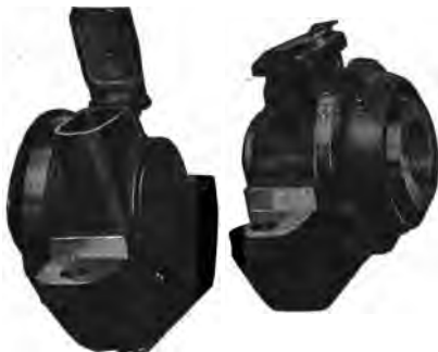
Figs. 3,527 and 3,528. —Frame heads for General Electric split frame motor. These heads are of the solid type and special provision is made to secure good lubrication.
