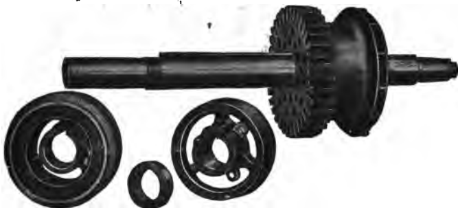
FIGS. 3,534 to 3,537. —Armature construction of General Electric ventilated railway motor. The core is built up of laminations mounted upon and keyed to the armature shaft. The armature is so constructed that the shaft can be removed without disturbing the windings or connections to the commutator. The laminations are punched and assembled with the holes in alignment so as to provide longitudinal holes through the core structure. The pinion end thrust collar has two oil throws, and the commutator end thrust collar, three, so designed as to prevent oil reaching the interior of the motor.
