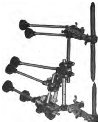
FIG. 3,878. Powers' arc lamp. Carrying capacity 100 amperes. All adjustments are accomplished from the outside of the lamp house. Carbon range from \frac{3}{8} " to \frac{3}{4} " in diameter, 6" length for lower and 12" length for upper carbon. The carbon may be placed at any angle desired, and can be moved independently of each other, forward, backward and sideways, or the whole lamp can be swung forward or backward, laterally, and up and down.
