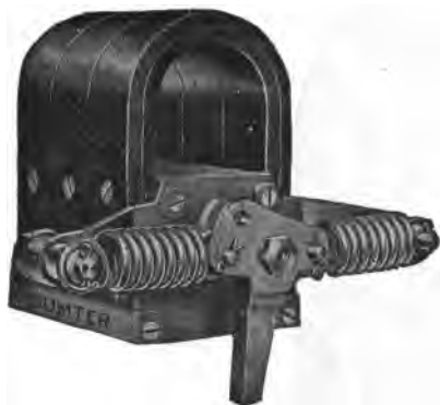
FIG. 3,960. —Sumter low tension oscillating magneto. In this type the armature does not revolve continuously but oscillates back and forth through an angle of about 90°.
