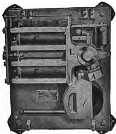
FIG. 3,677. —Safety Lighting Co., type F, lamp regulator. It consists of two piles of carbon discs in series with the lamps; the two piles being in parallel. The pressure on these carbons, and therefore their resistance, is determined by the armature of a magnet, the windings of which receive lamp voltage. By a unique design of magnet and levers, a high degree of accuracy in voltage regulation is accomplished without the use of any auxiliary control. The carbons C, are compressed by an adjustable spring connected to the link L, acting through a toggle. The pull of the spring is opposed by the pull of the electro-magnet which is connected directly across the lamp mains and is so designed that the armature A will stay in any position through its stroke when the lamp voltage is right. When the lamp voltage is high the magnet becomes stronger and pulls armature A down against the pull of the spring and reduces the pressure upon the carbons C, increasing their resistance and bringing the lamp voltage back to normal. If the lamp voltage be low, the magnet becomes weakened, the spring pulls armature A back, and through the toggle exerts enough pressure on the carbon piles to decrease their resistance and bring the lamp voltage back to normal. An air dash pot of the same type as used on the dynamo regulator is employed on the lamp regulator.
