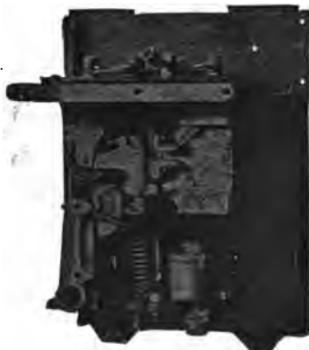
FIG. 3,636. —Westinghouse unit switch with sides of box, arc chute, cylinder and valve cut away. The construction of the switch includes two stationary copper castings, one of which forms directly the upper or fixed contact, while the other serves as a support for the lower or movable contact. The current carrying parts are enclosed in an insulating box of moulded material, in addition to which the jaws of the switch are further surrounded by an arc chute slipped inside of the switch box to protect the latter from the arc. The switch secured to the base plate of the switch group by two copper bolts, one of which is screwed into each of the stationary castings; and these same bolts serve as terminals to carry the current. By merely removing these two bolts the entire switch unit, complete with insulating box and arc chute, can be readily taken out. The force with which the switches operate is independent of the force with which the magnet valves operate. As long as the trolley voltage is sufficiently high to operate the magnet valves at all (200 volts), the switches close and remain closed with the same certainty and power as when the full normal voltage of 600, or more is available.
