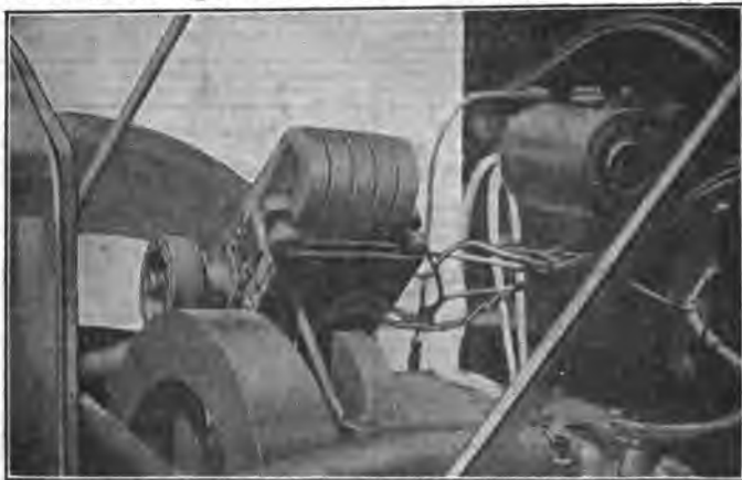
FIG. 4,030. —Method of driving a generator direct from engine fly wheel by friction pulley with spring or cushion base; the latter relieves the stress on the shaft from excessive vibration. The governor regulates the speed of the machine and prevents burning out of the lamps. The illustration shows a K-W magneto installed on an early Maxwell car.
