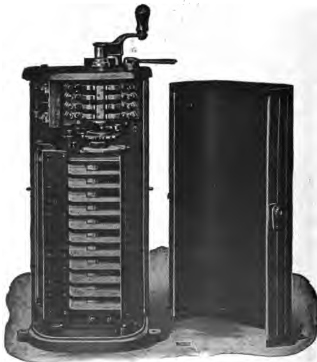
FIGS. 3,549 and 3,550. —General Electric series parallel controller. In this type, of which there are several forms, the power circuits are not broken during transition from series to parallel connections. The series parallel controller, as is well known, is used to control two motors, or two pairs of motor, and serves to connect these motors in series or in parallel relation. By means of these connections a car may be run economically at a medium speed, as well as at full speed, and can be accelerated to full speed more efficiently than is possible with a simple rheostatic controller. Hence, the practically universal adoption of the series parallel controller in railway service. The older forms of K controller were designed for operation on a normal line pressure of approximately 500 volts. With the advent of the commutating pole railway motor, the use of higher operating pressures, 600 to 650 volts, became possible and is now common practice, especially on interurban lines. To successfully operate on these higher voltages, individual blow outs and other features were introduced.
