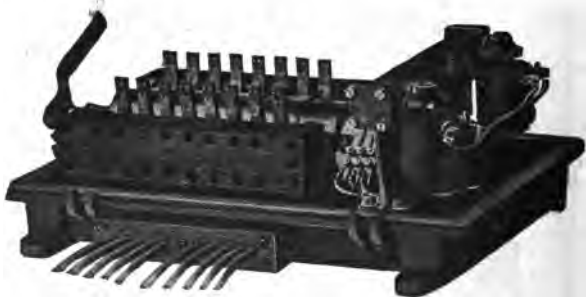
FIG. 3,641. —Westinghouse standard reverser, covers removed. The reverser comprises a number of copper fingers mounted on a stationary base, and pressing on one or the other of two sets of movable contact carried on a wooden drum. The drum is revolved to the forward or the reverse position by one or the other of two pneumatic cylinders, each controlled by a magnet valve similar to those in the switch group. Powerful forces approximating those for operating the switches, are used for moving the reverser, so that heavy pressures on the fingers and firm contacts are thus secured. This construction gives the reverser large overload capacity for taking care of heavy current rushes. No springs are used in the reverser cylinders and the drum, when moved to one position by closing the circuit of one of the magnets, remains in that position until the circuit of the other magnet is closed. Suitable small fingers mounted upon the reverser frame, and pressing upon corresponding movable contact pieces on the reverser shaft, establish the necessary interlocking connections. The reverser parts are built upon a skeleton cast iron frame and enclosed by removable sheet iron covers.
