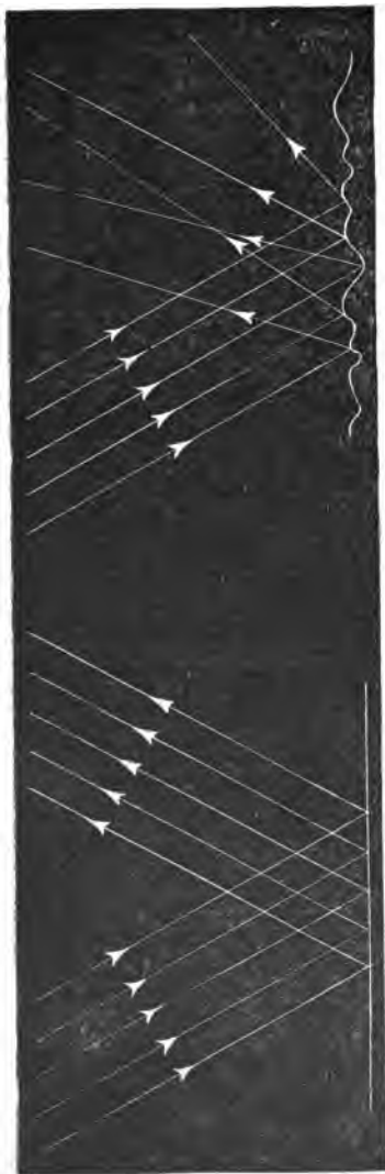
FIGS. 3,765 and 3,766. —Reflection from polished and unpolished surfaces. The difference between a smooth (polished) and a rough (unpolished) reflecting surface is here greatly exaggerated. In both cases the law of reflection for each ray of light is precisely the same, that is, the angle of incidence is equal to the angle of reflection . In the first case all portions of the reflecting surface are parallel to one another, and therefore reflect in the same direction all the rays which fall upon them from a given direction; in the second case, the elements of the surface are turned in a great variety of way and hence the reflected rays pass off in every direction. Even the smoothest surfaces which can be made diffuse light to a slight extent.
