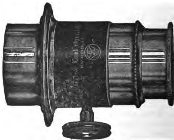
FIG. 3,814. —Bausch & Lomb standard projection lens. It consists of two combinations fitted into a cell and mounted in a brass tube which slides through a brass tube or sleeve. The focusing is by rack and prism, as shown. Connection is made for spherical and achromatic aberration. Equivalent focus 2\frac{1}{2} to 32 inches, and back focus 1\frac{1}{4} to 30 inches; corresponding diameter of lenses 1\frac{1}{8} to 2\frac{1}{4} .
