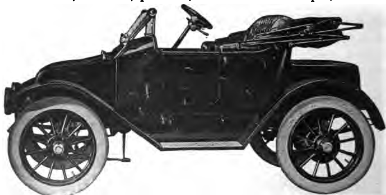
FIG. 4,058. —Baker electric roadster. The general specifications are as follows: frame, pressed steel; wheel base, 88 ins.; tread, 50 ins.; steering mechanism, two types, one with wheel steer, the other with lever steer; controller, continuous torque type, six speeds forward and three reverse; springs, semi-elliptic and full elliptic rear; battery, 34 cells, 13 MV thin plate Exide, standard; tires, 32×4 special electric pneumatic front and rear or 34×4 cushion front and rear; brakes, two sets of internal expanding on rear wheels, operated independently by two foot pedals; body aluminum, with side doors, open top, nickel and black metal finishings throughout; painting, body black, blue, green, or maroon panels, striping to match; upholstery, blue, green, or maroon leathers, or imported broadcloths, standard; fenders, full skirted metal curved fenders; equipment, two head lamps, two side lamps, tail lamp, side and storm curtains; volt ammeter and shaft odometer, full kit of tools, special adjustable clear vision wind shield, electric horn.
