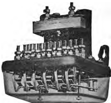
FIG. 3,727. —Polarized relay, wall type, with four front and four back neutral contacts and two front and two back polar contacts. The armature of this relay is itself a permanent magnet and swings back and forth to either pole of the electromagnet as the current attracts and repels it or whenever the polarity of the relay magnet changes.
