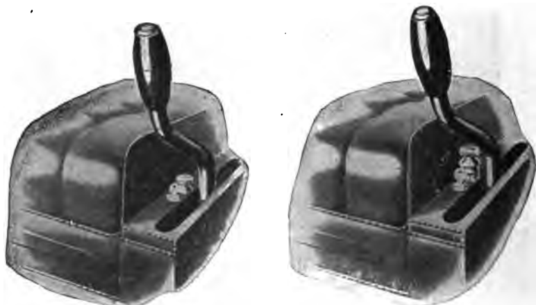
FIGS. 4,110 and 4,111 Broc control lever lock. Fig. 4,110, locked, safety plunger pushed down; fig. 4,111, ready to operate safety plunger raised. To unlock , insert and turn the key, move control lever back to power off position, and pull up safety plunger.
