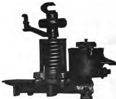
FIG. 3,637. —Westinghouse cylinder and magnet valve cut to show working parts. In operating the reaction of the spring, when compressed by the admission of air to the cylinder, is 120 pounds and the leverage is such that the pressure of 100 pounds appears at the switch jaws for forcing them apart. The same construction which secures the wiping action of the contact tips when the switch is closing is also of considerable benefit when it is opening, and an efficient application of the above force is obtained. The size of the air cylinder is such that the net pressure at the jaws for closing the switch is also approximately 100 pounds at all times of operation. The low voltage current from the trolley, through the control resistor, for operation of the valves is so small as to permit their arrangement for operation under a wide variation of trolley voltages. The assembled unit of cylinder and magnet valve is so secured to the frame of the switch group by means of two bolts that, like every other part of the group, it can be easily removed and replaced, should this become necessary.
