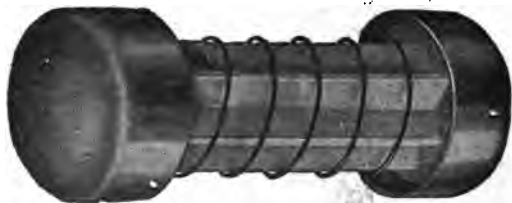
FIG. 4,057. —Rushmore ballast coil with cover removed to show the iron wire; illustration full size.
