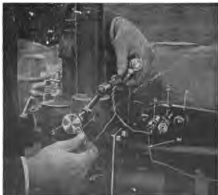
FIGS. 4,012 and 4,014.—Sumter testing device for testing low tension circuits. To test magneto, snap the clips on terminals after disconnecting it from circuit. The condition of magneto is evidenced by the brilliancy of lamp. To test a make and break ignitor, snap one clip on insulated terminal and the other on the engine frame. A little practice enables the conditions to be determined by noting the varying brilliancy of the lamp.
