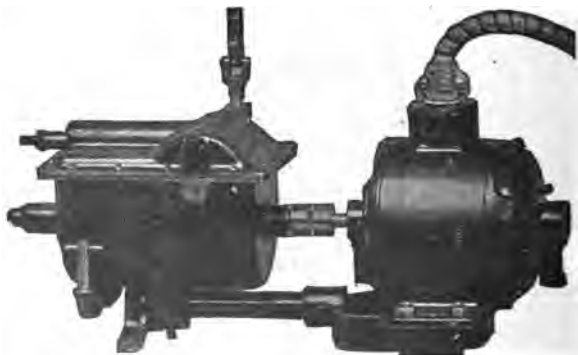
FIG. 3,885.—The arc controller or device designed to control the rate of feed of the carbons of an arc lamp, with the object of maintaining at all times a predetermined size of arc. It consists of the controller proper, direct coupled to a fractional horse power motor. There are two shafts, primary and secondary. The former, which is direct coupled to the motor, carries governor parts, and rotates constantly at the motor speed. The secondary, to which the telescope rod is geared, remains idle until the speed of the primary shaft exceeds the point of adjustment. The adjustment for any preferable size of arc is made with a brass adjusting nut upon a rod projecting from the cover of the controller. The inner end of the rod is connected through a heavy wire spring to a pawl, the function of which is to "step in" and transmit the power to the primary, through differential gearing to the secondary shaft, at the slightest tendency of the arc to become wider than the predetermined size adjusted for. The installation of the arc controller does not interfere with any of the lamp adjustments already provided. The operator may trim as he pleases, and feed by hand if he choose, by loosening a thumb screw at the feed handle gearing. Having loosened the thumb screw and trimmed the lamp, the operator strikes the arc by hand and makes the original and only feeding adjustment, by parting the carbons to the size of arc that he wishes to maintain; he then tightens thumb screw, and sets adjusting nut at the controller so that feeds do not occur below that size; the controller will then feed the carbons to that certain size of arc without further attention. To increase size of arc, tighten adjusting nut; to decrease size, loosen nut.
