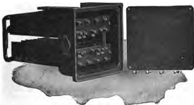
FIG. 3,645.—Westinghouse control resistor. This is used to reduce the trolley voltage for operating the magnet valves. The resistance element is of the slotted ribbon type, and is iron clad to protect it from the weather.
