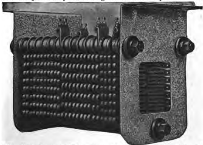
FIG. 3,642. —Westinghouse standard resistance grids for railway service. These grids are designed with the object of providing ample mechanical strength and liberal current carrying capacity. Individual grids of sufficient section to resist breakage are used; and this, together with the triangular arrangement of the tie rods, makes the assembled frames strong and solid.
