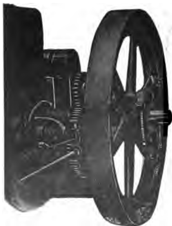
FIGS. 3,961 and 3,962. —Sumter low tension magneto installed on stationary engine, and marking on the ends of shaft and bearing for timing. To time , turn engine over in running direction until igniter snaps; be careful not to turn past this point. With gear on magneto shaft, turn the magneto in running direction until timing mark N on the shaft is in line with mark L, if rotation be left hand, or R, if rotation be right hand. Now mesh the gears, without moving the timing ; this is accomplished by a proper location of the keyway in the magneto gear in relation to a marked tooth on same. The teeth on the engine driving gear meshing with marked tooth on magneto gear should also be marked, and after this marking is once determined all keyways may be cut in proper relation to the marked tooth, thus making all magnetos on the same type of engine interchangeable. These magnetos are usually driven at engine speed, but may be driven at other speeds.
