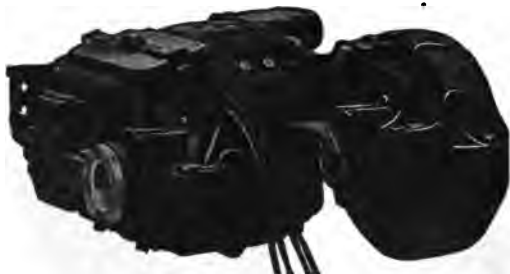
FIG. 3,541. —General Electric split frame motor. The frame is split horizontally with the suspension on the top half. The bottom half is arranged to drop to permit inspection of the interior of the motor from a pit. The armature bearing frame heads are of the solid head type giving the same qualities of oil lubrication as are obtained in the standard box frame motors. The upper and lower halves of the frame are held together by four bolts and two hinge bolts, and each frame head is firmly secured to the upper frame by bolts which are easily accessible from a pit. By removing these bolts (excepting the hinge bolts) and the lower half of the gear case, the armature can be removed. The upper and lower magnet frames are provided with machined surfaces fitting closely around the bearing heads, which act as keys in securing the alignment of the upper and lower halves of the motor frame. The axle bearing caps are bolted to planed surfaces on the top half of the frame and all the bolts are accessible from a pit. The armature is so constructed that the shaft can be removed without disturbing the windings or connections.
