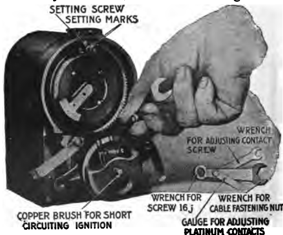
FIGS. 3,978 and 3,979. —Eisemann type G4 magneto showing method of timing and special wrench. Timing the magneto: As the spark occurs when the primary circuit is broken by the opening of the platinum contacts in the make and break mechanism, it is necessary that the magneto will be so timed that at full retard position of the timing lever body, the platinum contacts will open when the respective piston of the engine has reached the top point on the firing stroke. Turn engine by hand until piston of No. 1 cylinder is on the upper dead center; remove distributor plate from magneto and turn the driving axle of the armature until the setting mark on the distributor disc is in line with the setting screw as shown. (For clockwise rotation use mark R, for counter clockwise, use mark L). With the armature in this position, the platinum contacts are just opening, and the metal insert of the distributor disc is in connection with carbon for No. 1 cylinder. The driving medium must now be fixed to the armature axle without disturbing the position of the latter, and the cables connected to the spark plugs.
