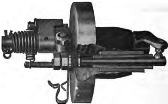
FIG. 3,966.—Sumter electrode for make and break ignition. In construction , the stem is insulated with rolled mica, which does not have any upturned edges in the combustion chamber. The taper arrangement makes it impossible to loosen or pull out the insulation. A copper gasket inside the igniter casting makes a gas tight joint. The stem is long enough to take care of igniter castings of various thickness, and the superfluous portion may be cut off.
