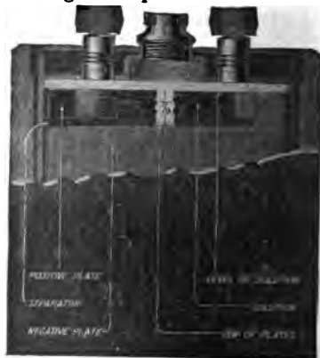
FIG. 4,088.—Sectional view showing height to fill Gould starting and lighting type of cell.
