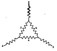
FIG. 1,379.— Diagram of six phasy winding consisting of combination of mesh and star grouping.
