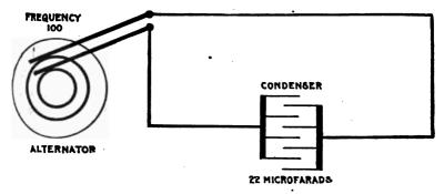
FIG. 1.287.—Diagram showing alternating circuit containing capacity. Formula for calculating the ohmic value of capacity or "capacity reactance" is  $X_{c} = 1 + 2\pi f C$ , in which  $X_{c} =$  capacity reactance;  $\pi = 3.1416$ ; f = frequency; C = capacity in farads (not micro-farads). 22 microfarads = 22 + 1.000,000 = .000022 farad. Substituting,  $X_{c} = 1 + (2 \times 3.1416 \times 100 \times .000022) = 72.4$  ohms.
