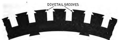
Pro. 1.478.—A style of disc largely used for armature cores. The teeth are provided with dovetail grooves near the circumference. After the coil is inserted in a groove, a wooden wedge is driven in the groove which encloses the coil and secures it firmly in position This obviates the necessity of bands to resist the centrifugal force acting on the inductors.
