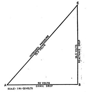
FIG. 1.321.—Diagram for impressed pressure on circuit containing 5 ohms resistance and inductance of 15 milli-henrys, the current being 10 amperes with frequency of 60.
