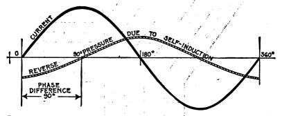
FIG. 1,308.—Sine curves showing phase relation between current and reverse pressure of selfinduction. This reverse pressure, being proportional to the rate of change in the current strength, is greatest when the current is at zero value, and zero when the current is maximum, and in phase is 90° behind the current.
