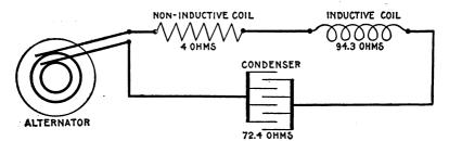
FIG. 1,300.—Diagram of circuit for example IV.
