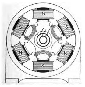
PIG. 1.528.—Diagram of six pole single phase alternator with concentrated half coil or hemitropic winding of same capacity as in fig. 1.527. There are an equal number of inductors, but in this case arranged in three instead of six coils. In this winding the direction of winding is alternately reversed so that the induced pressures do not oppose one another.
