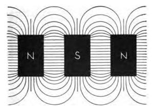
FIG. 1,426.—Diagram showing lateral field between adjacent poles.
