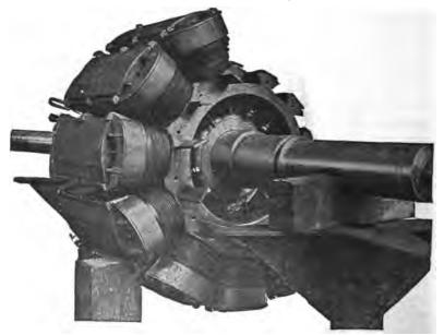
FIG. 1,466.—Wagner revolving field of 300 kilowatt alternator during construction, illustrating the method of attaching the field magnets to the hub by dovetail joints. After the notched ends of the pole pieces are slided into the grooves in the hub, tapered keys, which are plainly seen, are driven in, thus making a tight joint which will not shake loose.
