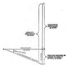
FIG. 1,337.—Impedance diagram of a circuit containing 25 ohms resistance, 30 ohms inductance, and 40 ohms capacity. The resultant reactance being due to excess of capacity, the impedance line AC' falls below the horizontal line AB, indicating that the current leads pressure.
