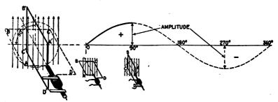
FIG. 1,222.—Diagram illustrating *amplitude* of the current. The current reaches its amplitude or maximum value in one quarter period from its point of zero value, as, for instance, while the generating loop moves from position ABCD to A'B'C'D'. At three-quarter revolution, the current reaches its maximum value in the opposite direction.
