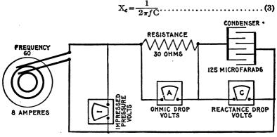
FIG. 1,330.—Diagram of circuit containing a resistance of 30 ohms and capacity of 125 microfarads. The calculation for impressed pressure, ohmic drop, and reactance drop for a current of 8 amperes at frequency 60 is given in the example on page 1,089, the diagram for impressed pressure being given in fig. 1,331.
