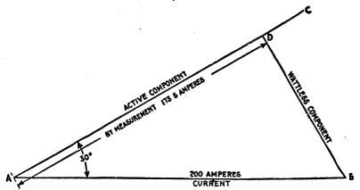
FIG. 1,359.—Diagram for obtaining the active component of the current in a circuit having a current of 200 amperes and angle of lag of 30°.
