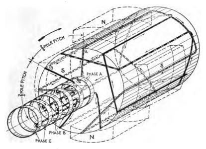
FIG. 1,374.—Elementary four pole three phase alternator. There are three sets of inductors, each set connected in series and spaced on the drum with respect to each other two-thirds pole pich apart. As shown, six collector rings are used, but on actual three phase machines only three rings are employed, as previously explained. The inductors have distinctive coverings for the different phases. The arrows indicate the direction in which the induced pressures tend to cause currents.
