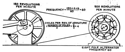
FIG. 1,223.—Diagram of alternator and engine, illustrating frequency. The frequency or cycles per second is equal to the revolution of armature per second multipled by one-half the number of poles per phase. In the figure the armature makes 6 revolutions to one of the engine; one-half the number of poles = 8 + 2 = 4, hence frequency =  $(150 \times 4 \times 6) + 60 = 60$ . The expression in the parenthesis gives the cycles per minute, and dividing by 60, the cycles per second.
