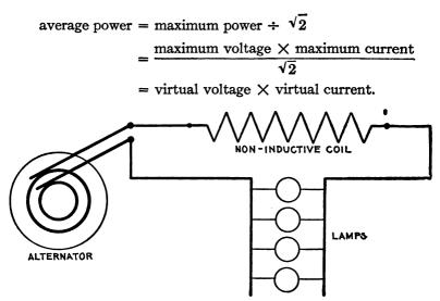
FIG. 1,347.—Diagram of circuit containing only resistance; in such a circuit the power factor is unity.
