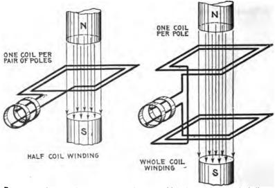
FIGS. 1,488 and 1,489.—Elementary bipolar alte nators with half coil and whole coil windings. In a half coil winding there is one coil per phase per pair of poles; in a whole coil winding there is one coil per phase per pole.
