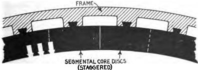
FIG. 1.480.—Construction of large stationary armature; view showing section of core and frame. The core discs are in segments and are attached to the frame by dovetail joints as shown. The joints are staggered in building up the core, that is, they are overlapped so as not to unduly increase the reluctance of the magnetic circuit. Dovetail joints obviate the use of through bolts which, if not insulated, are liable to give rise to eddy ourrets by short circuiting the discs.
