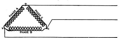
**FIG. 1.549.**—Diagram of three phase mesh grouping, commonly called delta grouping owing to its resemblance to the Greek letter  $\Delta$ . The voltage at the terminals is equal to the voltage in one phase, and the current in each line is equal to the vector sum of the currents in two phases, that is, it is equal to  $\sqrt{3}$  multiplied by the current in one phase.
