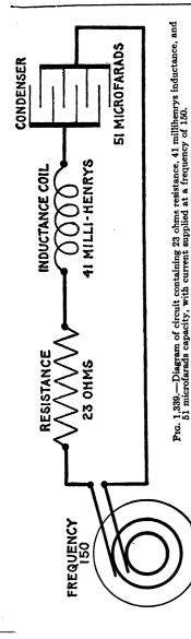
EXAMPLE.—A current has a frequency of 150. It passes through a circuit, as in fig. 1,339, of 23 ohms resistance, of 41 millihenrys inductance, and of 51 microfarads capacity. What is the impedance?
