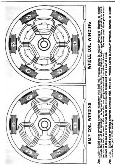
all the turns of the coil are placed in single slots, the winding is called "concentrated."
