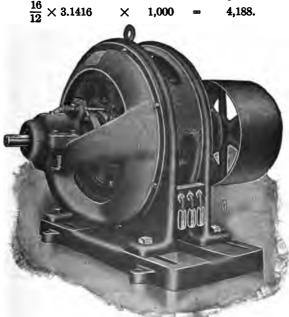
FIG. 1,384.—Fort Wayne revolving field belt driven alternator. It is designed for belted exciter, having a shaft extension at the collector ring end for exciter driving pulley.
