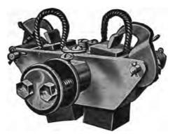
FIG. 1,561.—Triumph brushes and brush holder. The holder is of the box type provided with an adjustable tension spring, making the brushes self-feeding. Each holder is carried on insulated studes attached to a cast iron yoke which is mounted on the bearing.
