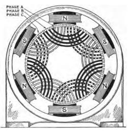
FIG. 1.536.—Three phase winding with distributed coils—wound in four slots per pole per phase; diagram showing placement of the coils.
