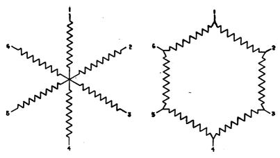
FIG. 1,376.—Diagram of six phase winding with star grouping, being equivalent to a three phase winding in which the three phases are disconnected from each other and their middle points united at a common junction.
