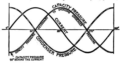
FIG. 1.328.—Current and pressure curves, showing phase relation between the current, condenser pressure, and impressed or *capacity* pressure necessary to overcome the condenser pressure. The capacity pressure, since it must overcome the condenser pressure, is equal and opposite to the condenser pressure, that is, the phase difference is 180°. The condenser pressure being 90° *ahead* of the current, the impressed pressure is 90° *behind* the current.
