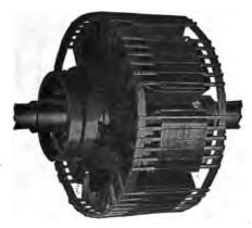
FIG. 1,405.—Westinghouse field with amortisseur or "damper" winding for 75 kva. and larger beited alternators, which prevents hunting and reduces eddy currents in the pole pieces. The copper bars of the amortisseur cage winding are arranged in partially closed slots in the pole pieces.
