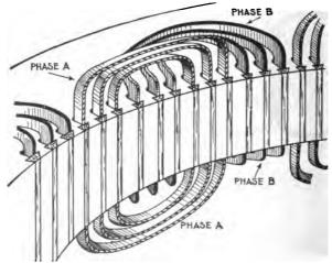
FIG. 1.534.—Section of two phase winding showing shaping of the coil ends. Every other coil is flat, while the alternates have their ends bent down as shown. With respect to the shaping of the coil ends, it is called a *two range winding*.
