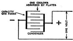
FIG. 1,281—Diagram illustrating a *farad*. A condenser is said to have a capacity of one farad if it will absorb one coulomb of electricity when subjected to a pressure of one volt. The farad is a very large unit, and accordingly the microfarad or one millionth of a farad is often used, though *this must be reduced to farads before substituting in formula*.
