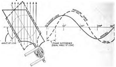
FIG. 1,289.—Pressure and current curves illustrating *lead*. The effect of capacity in a circuit is to cause the current to rise to its maximum value sconer than it would otherwise do; capacity produces an effect exactly the opposite of inductance. The phase relation between current and pressure with current leading is shown graphically by the two armature positions in full and dotted lines, corresponding respectively to current and pressure at the beginning of the cycle.
