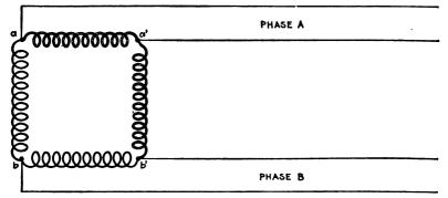
FIG. 1,545.-Diagram of two phase mesh grouping.
