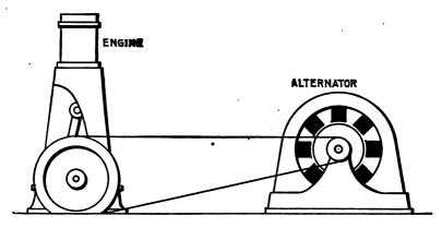
FIG. 1,380.—Belt-driven alternator. By use of a belt, any desired speed ratio is obtained, enabling the use of a high speed alternator which, being smaller than one of slow speed, is cheaper. It affords means of drive for line shaft and has other advantages, but requires considerable space and is not a "positive" drive. Belting exerts a side pull which results in friction and wear of bearings. Means for tightening the belt as shown in fig. 1,381, or equivalent, must be provided.
