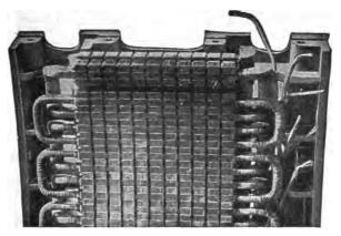
FIG. 1,487.—Section of General Electric stationary armature ventilating ducts and winding in position.
