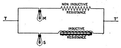
FIG. 1,265.—Non-inductive and inductive resistances. Two currents are shown joined in parallel, one containing a lamp and non-inductive resistance, and the other a lamp and inductive resistance. The two resistances being the same, a sufficient direct pressure applied at T, T' will cause the lamps to light up equally. If, however, an alternating pressure be applied, M will burn brightly, while S will give very little or no light because of the effect of the inductance of the inductive resistance.
