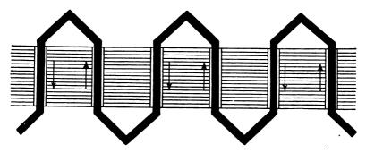
FIG. 1,526.—Developed diagram of a single phase monotooth or one slot bar winding; it is suitable only for operation at low voltage.
