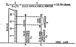
FIG. 1,335.—Impedance diagram for circuit (of above example) containing inductance and capacity. With any convenient scale, erect a perpendicular AB = 18.25 ohms, and CD = 12.76 ohms. Continue CD by dotted line to D' so that CD'=AB, then DD'=AB - CD = inductance reactance -capacity reactance, which is equal to the impedance. Expressed by letters  $Z = X_4 - X_c = DD'$ , which by measurement = 5.49 ohms.
