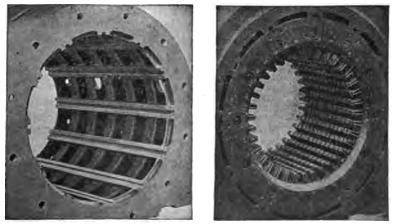
FIGS. 1,575 and 1,576—Westinghouse turbine alternator armature construction. Fig. 1,575. View showing dovetail grooves in armature casting; fig. 1,576, laminae assembled in dovetail grooves of armature casting.
