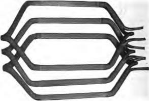
FIG. 1,504.—Allis-Chalmers lap wound coils torming a three slot distributed coil unit. In construction, after the coils have been covered with insulating materials and treated with insulating compound, the parts that lie in the slots are pressed to exact size in steamheated moulds. This runs the insulating material into all the small spaces in the coil, excluding moisture and rendering the insulation firm and solid. The ends of the coils, where they project beyond the slots, are heavily taped.
