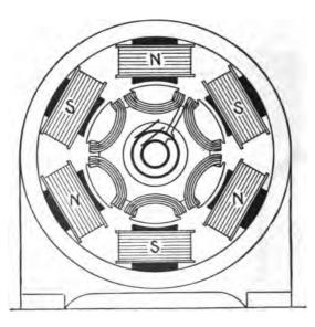
FIG. 1,527.—Diagram of six pole single phase revolving armature alternator, with monotooth or concentrated whole coil winding. For 3,000 volts at 900 revolutions per minute, 120 inductors are required. And in the case of a concentrated or monotooth winding they may be arranged in "whole coils" as above or in "half coils" (hemitropic) as in fig. 1,528.
