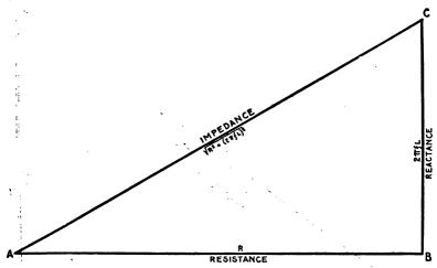
FIG. 1.322.—Graphical method of obtaining the impedance in circuits containing resistance and inductance, having given the resistance and reactance, that is. the obmic resistance and spurious resistance. With any convenient scale lay off AB = resistance, and erect the perpendicular BC = reactance (using the same scale); join AC, whose length (measured with the same scale) will give the impedance.
