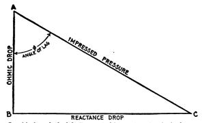
Fig. 1.319.—Graphical method of finding angle of lag when the ohmic drop and reactance drop are given. The angle of lag  $\phi$ , is that angle included between the impressed pressure and the ohmic drop lines, that is, between AC and AB.
