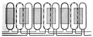
FIG. 1,550.—Three phase winding with short coils. The use of short coils as here shown, in which the coil breadth = 36 pole pitch, avoids the necessity of overlapping.
