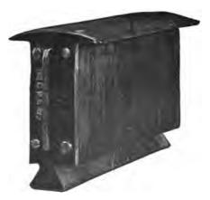
FIG. 1,465.—Wagner lamins.ted pole plece with horns stamped in one piece. The laminations are held together between two end pieces by through rivets, as shown.
