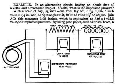
FIG. 1,316.—Diagram of circuit containing 5 volts ohmic drop, and 15 volts reactance drop.
