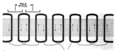
FIG. 1,501.—Developed diagram of single phase concentrated whole coil winding in two slot stamping for six pole alternator. If the sides of adjacent whole coils be slightly separated by placing the winding in a two slot stamping the electrical result will not differ materially from the monotooth whole coil winding, but if the winding be hemitropic, as in fig. 1,502, and has coils of two sizes as shown, it will be suitable for high voltages.
