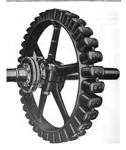
FIG. 1.463.—Triumph 36 pole fly wheel type revolving field. The spider has the form of a fly wheel having spokes and rim to which the field magnets are attached by through boks. The field coils are of copper strap bent on end, the kind generally used on large machines. The series connection of the coils is plainly shown, also the two cables leading via one of the spokes to the slip rings.
