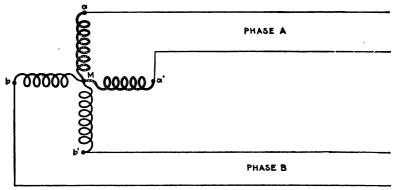
FIG. 1,544.-Diagram of two phase star grouping.
