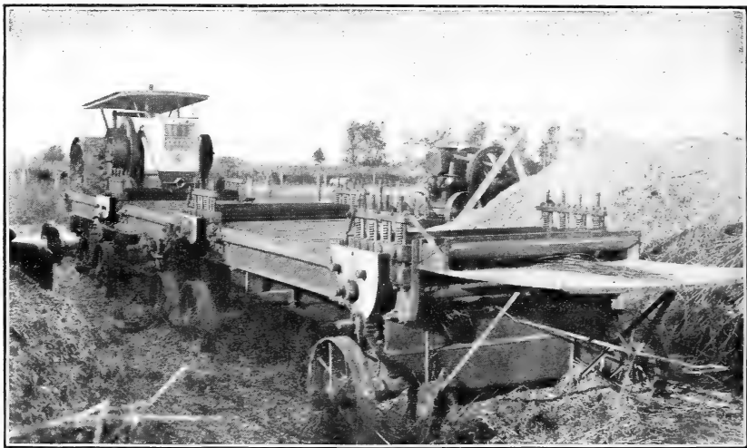
FIG. 2.—Machine brake and hemp hurds. Hemp hurds from machine brakes quickly accumulate in large piles.
