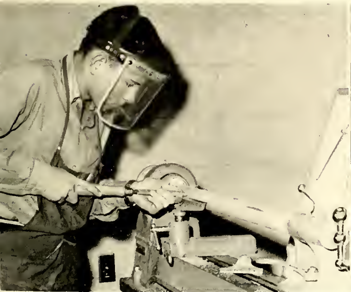
IN SHOP Gene Wright works skillfully as he turns a table leg on a lathe.
