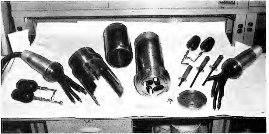
Figure 12. Components of the prototype wet connector.
