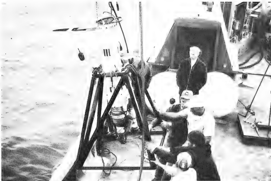
Figure 20. Connector and remote mating equipment used during deep ocean test at 4,000 feet.
