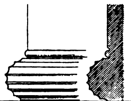
FIG. 48.—Base from the porch of the Gabre, Pasargadæ. Profile and section. FLANDIN and COSTE, Perse ancienne , Plate CLXXVII.
