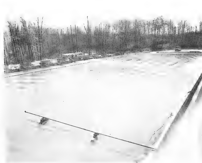
Figure 38. Waves being generated in the shore processes test basin. The 10 wave generators could be operated independently or synchronized electronically to operate as a single, long generator.
