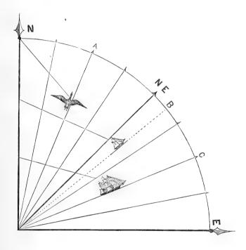
points of the wind; B is the course of a cutter which can sail 'close hauled' to within four points and a half of the wind; A is the course of the Albatross, which flies so close to the wind as to keep within two points of the wind, and appears almost to fly against it."
