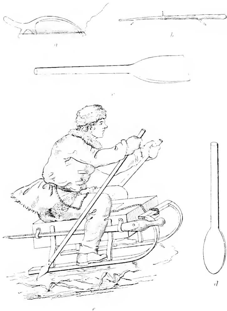
Fig. 8. Fishing-tackle used in winter: a and b : rods, c and d : ice-shovels, e : fishing-sled, with ice-chisel fastened at the side.
