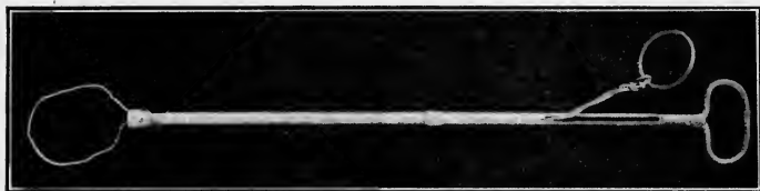
PLATE 17. Convenient hog holder made from \frac{1}{2} inch gas pipe and flexible clothes wire. It may be disjoined in the middle for convenience in carrying
