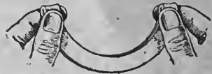
Fig. 11. A simple method for testing rubber rings for jars. Fold the ring and press tightly and then turn it over and reverse the fold in the same place. A perfect rubber for Cold-pack canning will show no crease or break after this has been repeated two or three times.
