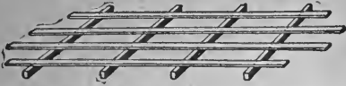
FIG. 1. Home-made rack for placing in wash-boiler for holding jars. The cross pieces should be thick enough to allow circulation of water underneath jars.
