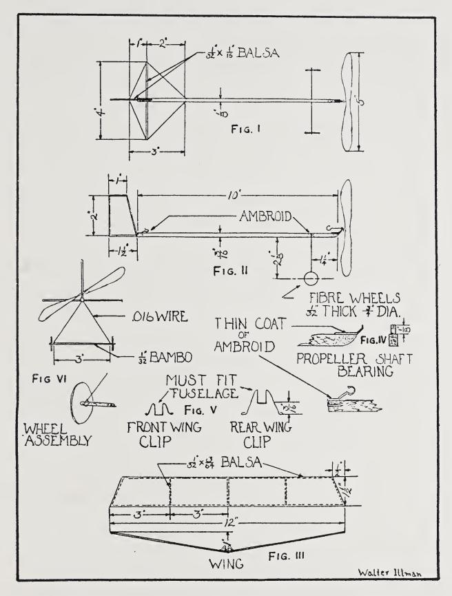
light pamphlet is laid on the other which is lying flat on the drawing. Apply ambroid at the two cuts and leave the frame unmolested until it has dried. The wing now looks like a flat V; this is called a
