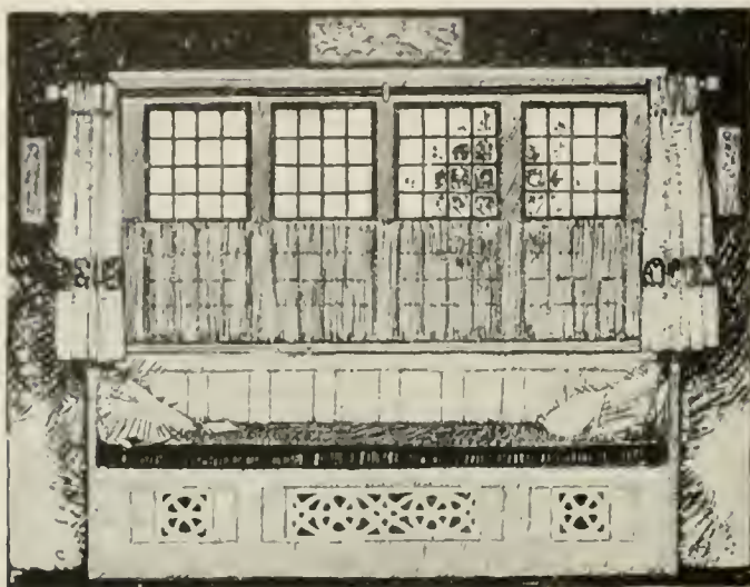
In this drawing note the method of screening the radiator which is under the seat. Note also the picturesqueness of the window arrangement with its small panes and simple hangings.
