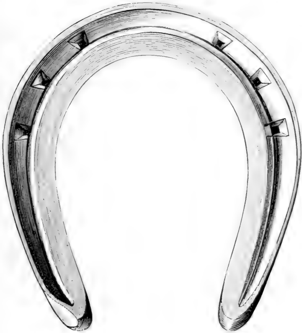
Fullered and seated-out shoe.
