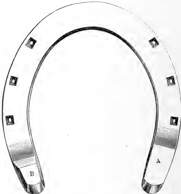
B—Calkin turned up narrow. Under inner posterior edge of toe not rounded off.
