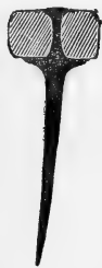
Fig. 163. Section of the head of a garden-rake, showing how the teeth should be inserted in it.
