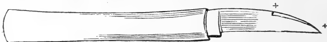
Fig. 195. Grafting-knife, with the portion of the back of the blade from + to + ground to a cutting edge, so as to make it serve also for a budding knife.
