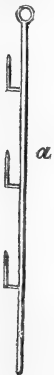
Fig. 266. Wire-standard for supporting rings, so as to form the frame-work shown in fig. 264.
