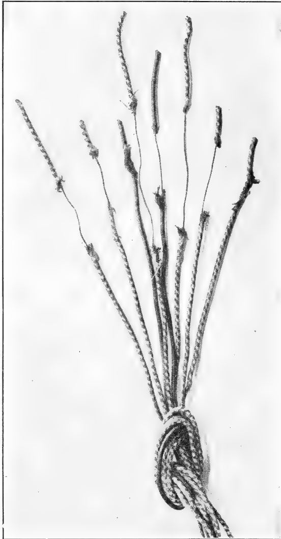
FIGURE 7.—Rat damage to wires explains some interruptions to telephone service.
