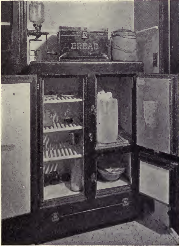
FIG. 132.—Refrigerator showing good interior arrangement.
