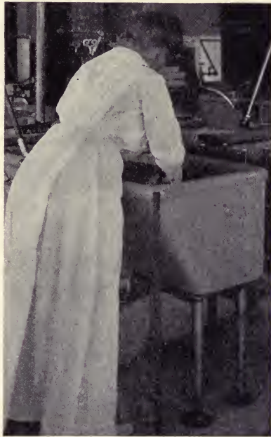
FIG. 63.—The top of this tub is 36 inches from the floor. Note good position of worker's back.
