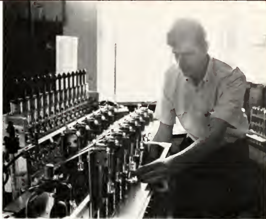
A grad student measures oxygen uptake of tissues in a differential respirometer.
