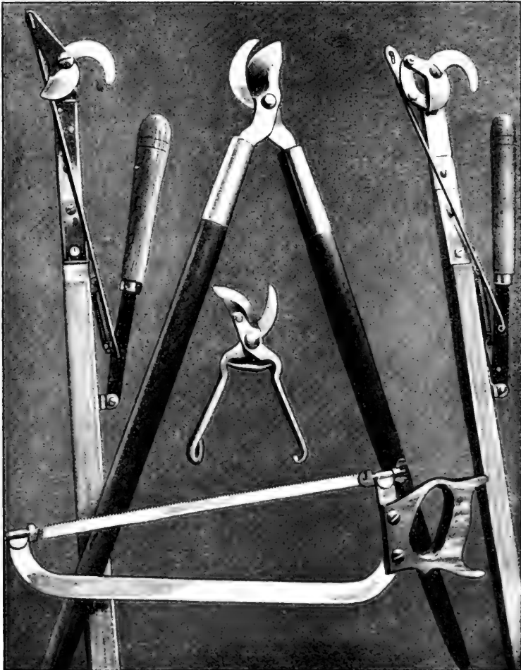
Good pruning tools. Note wide open hand shears, and pole pruner—both double action.
