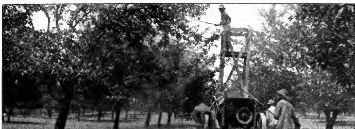
Note the tower on wagon frame, and the long nozzle rod for high limbs.
