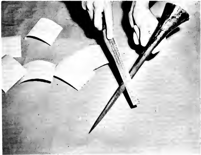
Fig. 156. Sailfish and marlin bills make unusual and attractive letter openers. File and sand the upper and lower (dorsal and ventral) sides.
