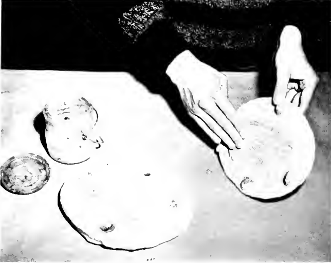
Fig. 73. The first step in casting the fins is to apply the wax-kerosene separator. Rub it well into the mold with your fingers.
