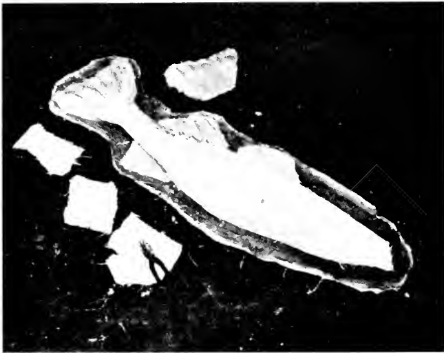
Fig. 63. Medium and large fishes require stronger casts. This is accomplished by backing the first layer of plastic in the mold with glass (woven glass) and an additional plastic layer of plastic.
