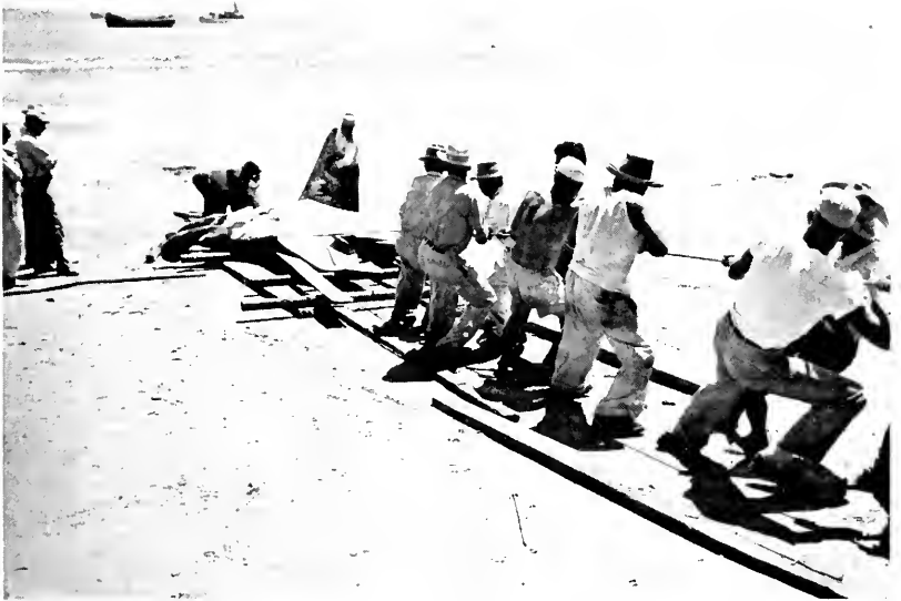
Fig. 168. Planks and rollers were placed under the manta. A rope was tied to a truck, and everyone pulled.
