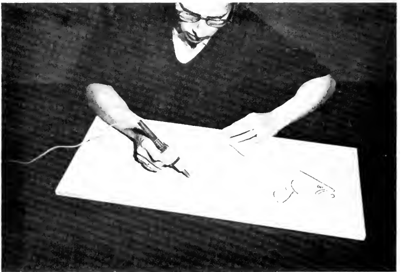
Fig. 124. Burn the outline into the wood with an electric "wood burning pen."
