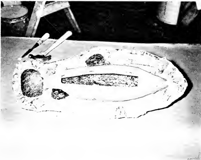
Fig. 59. Separate the halves of the mold by inserting a chisel between them. The cast will remain in one side.
