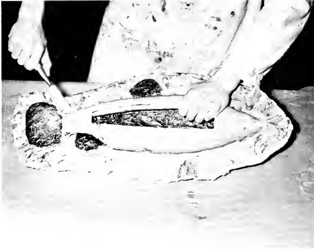
Fig. 61. Apply downward pressure on the chisel and the cast should come out.
