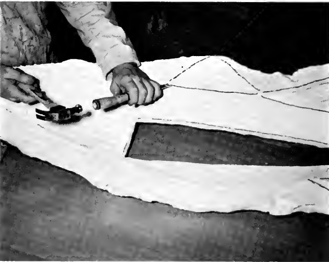
Fig. 42. Chip away the fin areas to a depth of about \frac{1}{2} inch.
