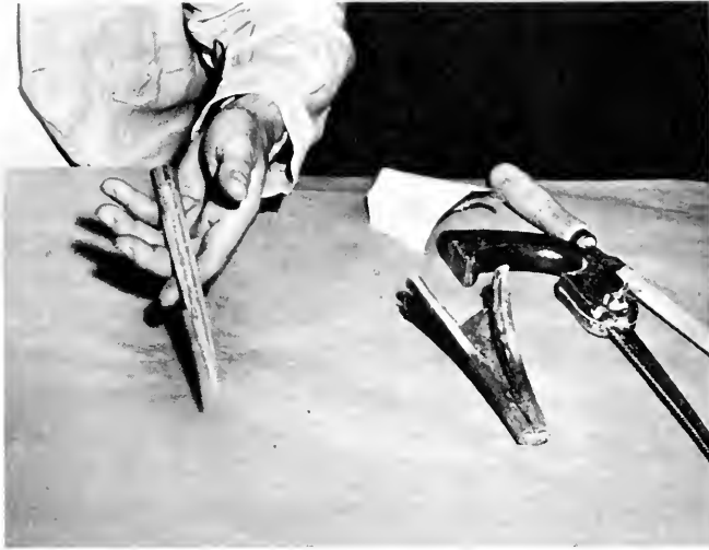
Fig. 157. Cut the base of the bill away from the solid front portion. Polish and add a handle.
