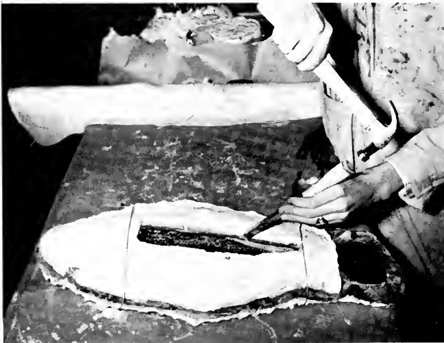
Fig. 58. The first step in removing the cast from the mold is to chip away any plastic which may have flowed over the edge of the back opening of the mold.
