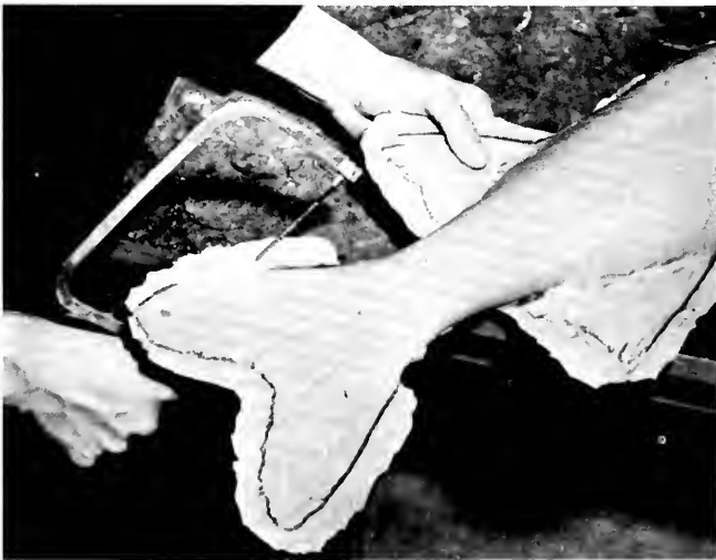
Fig. 68. Cut the excess material from around the fins.
