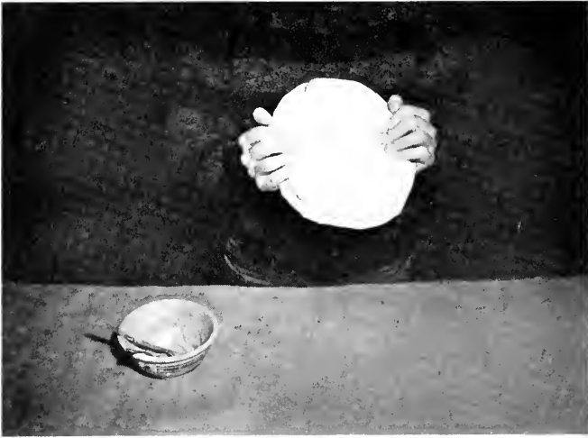
Fig. 75. Employ steady pressure so that the mold halves come together slowly.
