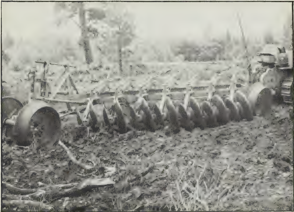
Figure 6. The Brushland plow killed practically all of the brush and prepared a good seedbed on this sagebrush area in the ponderosa pine zone in southwestern Colorado. The plow went over rocks, brush, and small trees without breaking or clogging. After plowing, the seedbed was allowed to settle until fall when it was drilled
