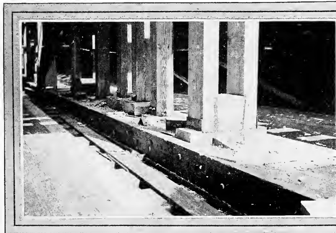
FIG. 154—DETAIL OF STANCHION FOOTINGS IN A LARGE WOODEN SHIP. FIG. 155—GENERAL VIEW OF STANCHIONS IN THE SAME SHIP
