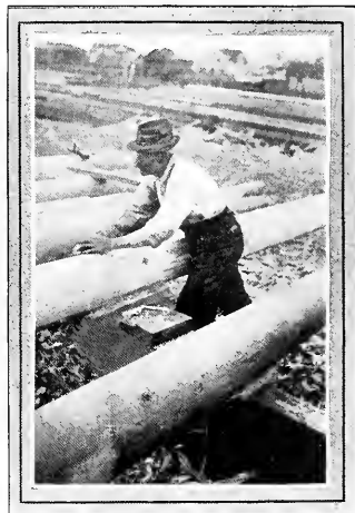
FIG. 187—FINISHING A SPAR WITH A HAND PLANE
