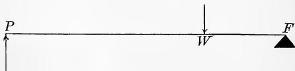
FIG. 64.—A lever of the second order. F , fulcrum; P , power; W , weight. The arrows indicate the direction in which the forces act.
