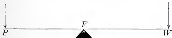
FIG. 36.—A lever of the first order. F , fulcrum; P , power; W , resistance or weight.
