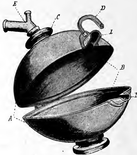
FIG. 117.—Roy's oncometer (open and empty), for study of variations in volume of the kidneys. Metal box, of approximately the same shape as the kidney, which opens by a hinge. Each half of the box contains two chambers, an outer A , and an inner B . The two upper chambers, from the top of which the two-way tube E passes out, are clamped together by screw C . The lower chambers are clamped by a similar screw. The box closes by the hook D , which surrounds the hollow tube L , through which the renal vessels and the ureter pass out from the enclosed kidney.
