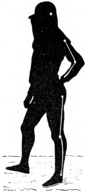
FIG. 77. — Subject wearing black clothes to obtain diagram of walking. Chronophotographic method. (Marey.)
