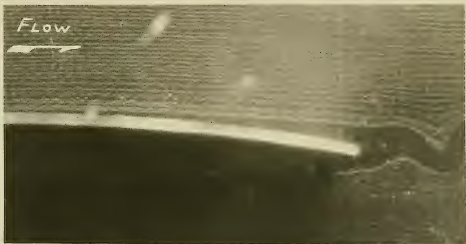
Figure 14 - Streakline Pattern About a Foil Shape, Aspect Ratio is 10:1 (Freestream Velocity is 1 fps)
