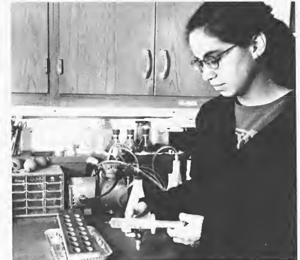
Pamela Templer extracts pore water from a sampling device called a peeper.
