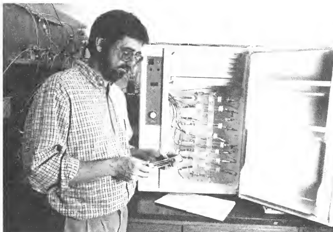
Dr. Verchot developed the apparatus he uses to measure denitrification. Here he holds one of the glass tubes in which soil samples are incubated.
