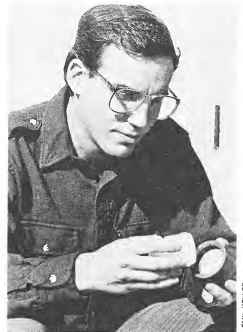
Gary Lovett examining a filter holder which will trap pollutants for analysis.
