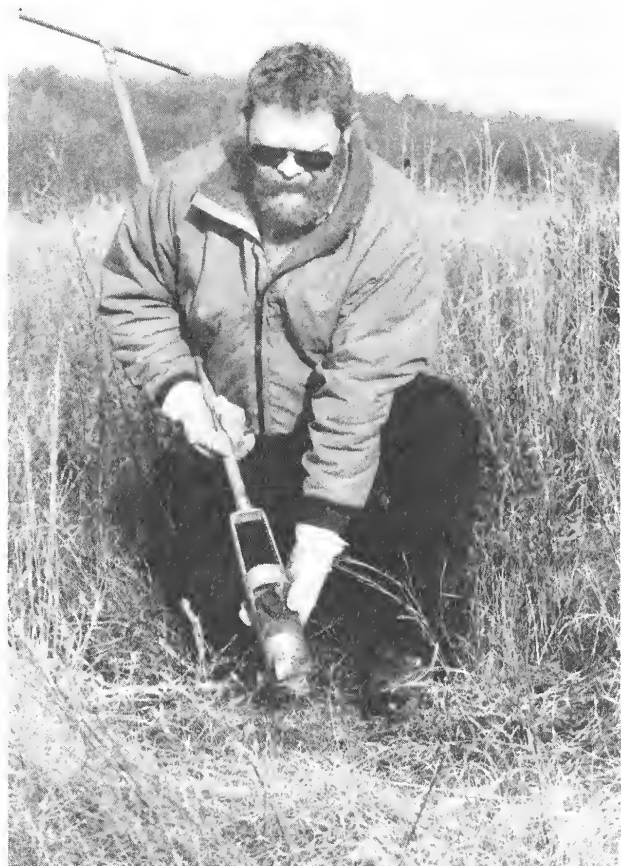
Dr. Joseph Boyer uses a soil auger to collect soil samples in different land use areas. He is comparing forested and agricultural sites to learn what factors affect denitrification.
