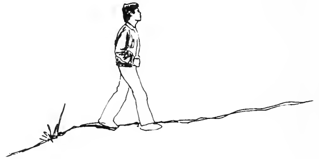
Figure 10. Pacing a distance on moderate slope. Count 1, 2, 3, 4, 5, 6, 7, 8, 9, 10, 10, 11, 12, 13, 14, 15, 16, 17, 18, 19, 20, 20...etc.
