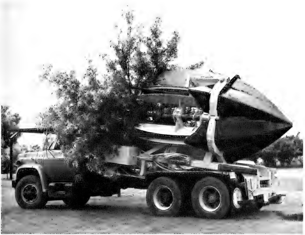
This large tree spade digs a soil ball 7 feet in diameter weighing about 4 tons, and it is capable of transplanting trees with trunks 6–8 inches in diameter. (Photo courtesy of Vermeer Manufacturing Co.)
