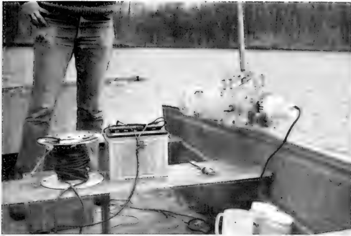
Submersible vacuum pump collecting equipment with battery in boat (Photo by John Barlow, Aquatic Biologist).
