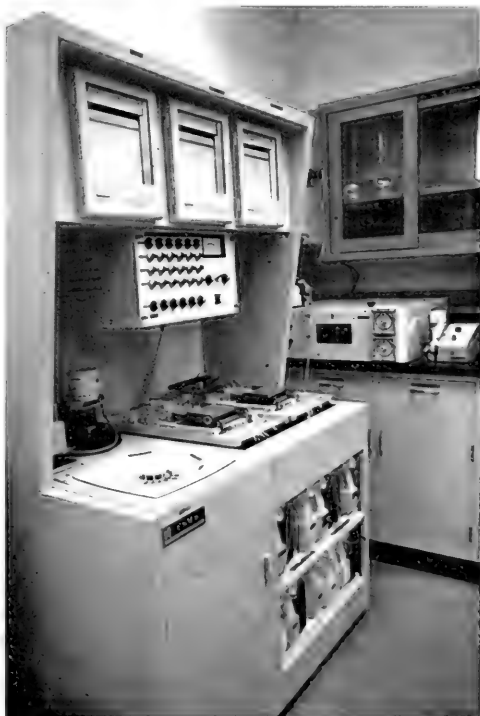
An automated analyzer which is capable of making multiple water analyses without operator attention. (Photo by former Survey photographer Wilmer Zehr.)
