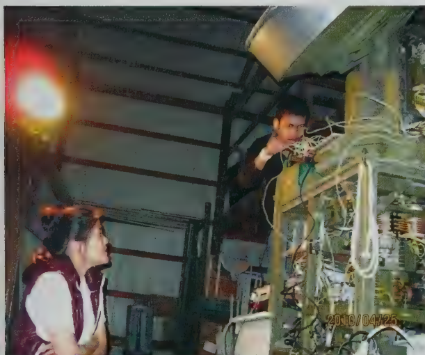
Two UIUC Electrical and Computer Engineering students fine-tune the INHS Doppler radar unit. Photo by Ron Larkin, INHS
