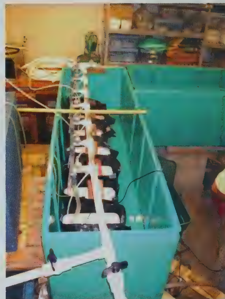
Photo 1. Experimental set up. Individual containers hold one largemouth bass each and heated/chilled water or oxygen/nitrogen is pumped into the containers to create the temperature and dissolved oxygen changes.
