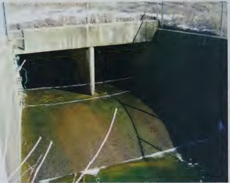
A PIT tag antenna at Lake Sam Dale, Illinois. Photo by Max Wolter, INHS
