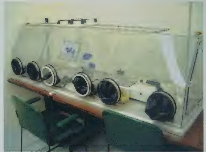
Glove box used to separate blood-fed from unfed female mosquitoes and to dissect blood-fed mosquitoes that survive the 14-day virus incubation period. Photo by Ephantus Muturi
