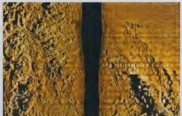
Figure 3. Sidescan sonar waterfall display showing areas of massive fractured bedrock dropping down to a smooth rippled sand substrate (upper right portion of the image) along the southern flank of Julian's Reef.
