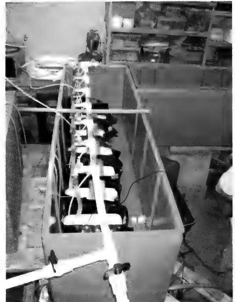
Photo 1. Experimental set up. Individual containers hold one largemouth bass each and heated/chilled water or oxygen/nitrogen is pumped into the containers to create the temperature and dissolved oxygen changes.
