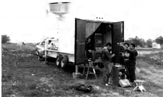
Three ECE students and an engineer aim a mechanized platform they created to point a night-vision imager in three dimensions. Photo by Ron Larkin, INHS
