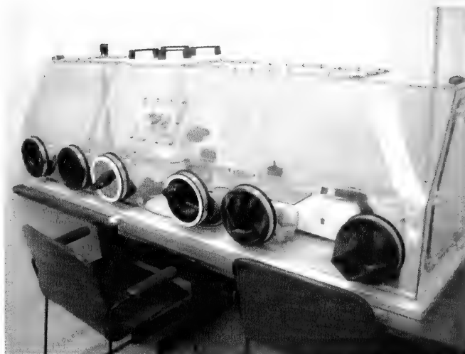
Glove box used to separate blood-fed from unfed female mosquitoes and to dissect blood-fed mosquitoes that survive the 14-day virus incubation period. Photo by Ephantus Muturi
