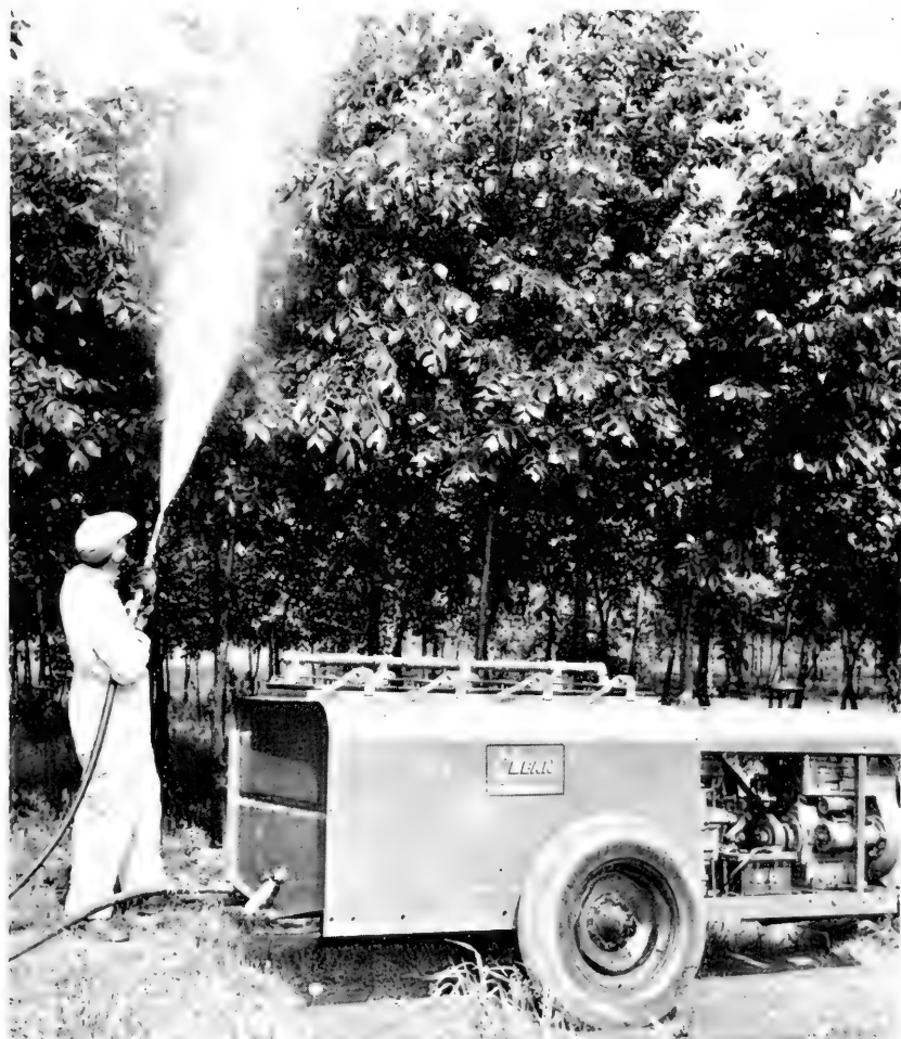
Fig. 65.—Hydraulic sprayers used in spraying elms with DDT for the control of the insects that carry Dutch elm disease or phloem necrosis must have sufficient power to give adequate coverage of the trees.
