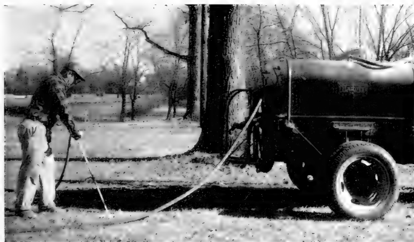
Fig. 31.—Hydraulic sprayers that develop several hundred pounds pressure can be used in liquid feeding of trees.
