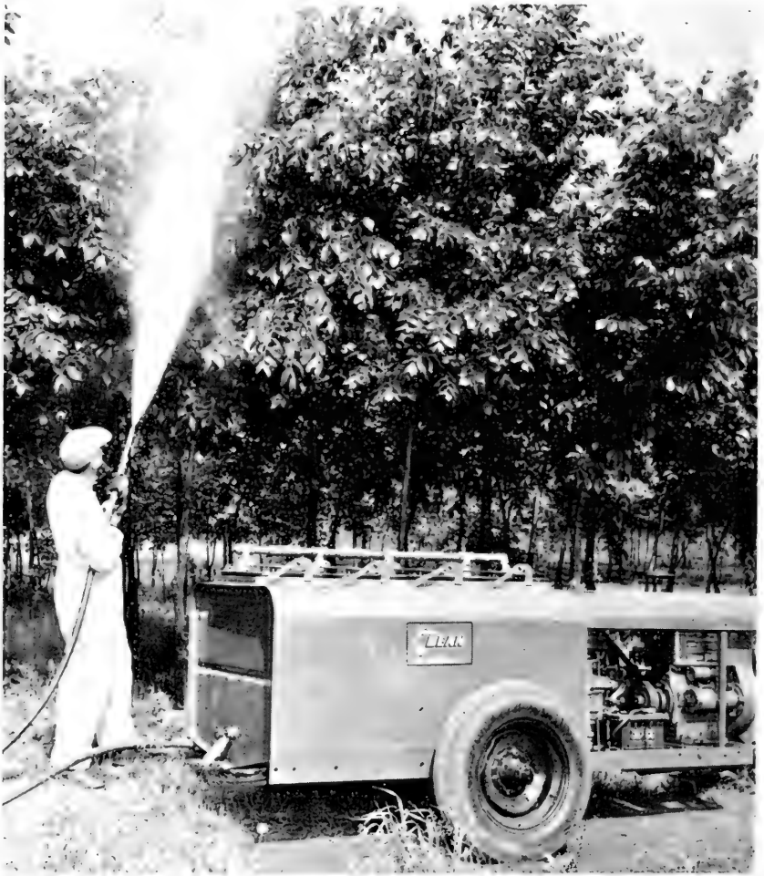
Fig. 49.—Hydraulic sprayers used in spraying elms with methoxychlor or DDT for control of the insect that spreads phloem necrosis must have sufficient power to give thorough coverage of all parts of trees. Drenching that results in excessive run-off should be avoided.
