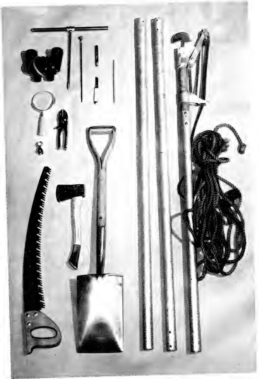
Fig. 28.—Tools useful in examining trees for diseases include knife, hand shears, saw, hatchet or ax, reading glass, hand lens, extension pruner, punch, increment borer, field glasses, and shovel.
