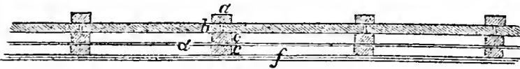
Fig. 61.— Hollow Walls for a Poultry House— a., Outside Battens ; b., Outside Boarding ; c., Middle Battens ; d., Felt ; e., Inner Battens ; f., Lath and Plastering .
