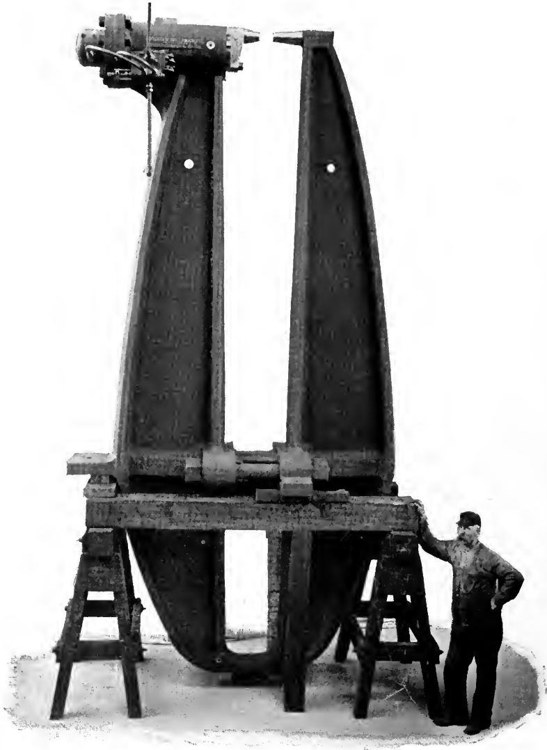
11 FT. HYDRAULIC RIVETER.
