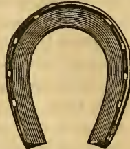
A FULLERED SHOE. (Ground surface.)
