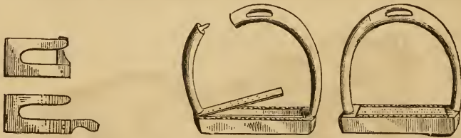
SPRING BAR FOR THE STIRRUP LEATHER AND SPRING STIRRUP. BOTH BEING EXHIBITED DURING REST AND WHEN IN ACTION.
