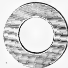
Ring used as an adapter for fitting various sized basins to the simple water bath. p. 93.
