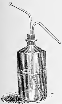
Wash bottle for washing precipitates. &c. p. 93.
