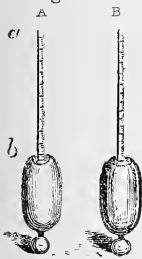
Urinometers for ascertaining the specific gravity of fluids. p. 93.
