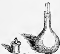
Bottle for finding the specific gravity of fluids by weight. p. 93.
