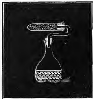
Flask adapted for the estimation of carbonic acid gas, used in determining the proportion of sugar in fluids by the fermentation test. p. 252.
