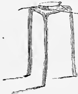
Wire triangles for supporting platinum capsules or foil while the organic matter is being burned off. p. 92
