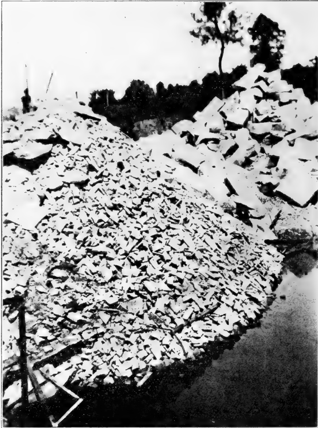
A large pile of mill waste at the plant of the Star Stone Company in Hunter Valley. This material could be used in a fine crusher without preliminary breaking. The pile in the background is quarry waste.
